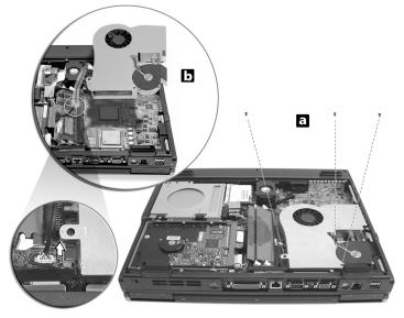
b) Unplug the air baffle power connector from the system main board and remove the air baffle/heat sink assembly to expose the CPU socket.
